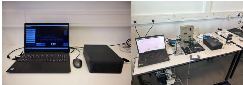
Figure 2-13: left: RAMASCOPE detection system. Right: Installation of RAMASCOPE on the testing table
