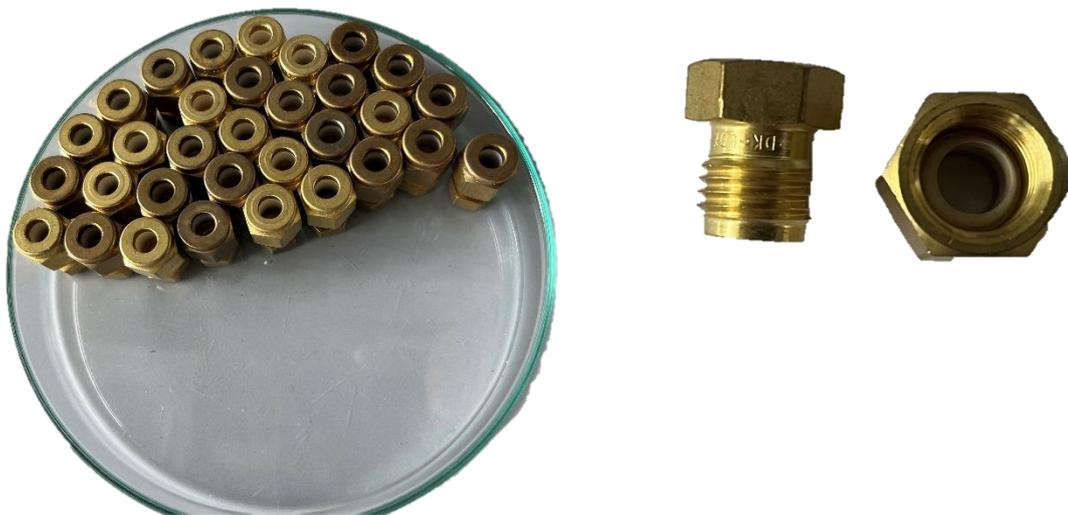
**Figure 3.5:** Unscrewed Coated brass compression caps (right). The unscrewed caps screwed together again, and prepared for heating in an oven (left).
