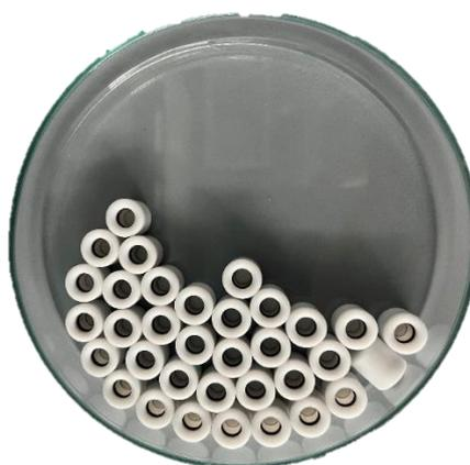
**Figure 3.6:** The rinsed Teflon caps with ethanol 70 %, preparing for heating in an oven.
