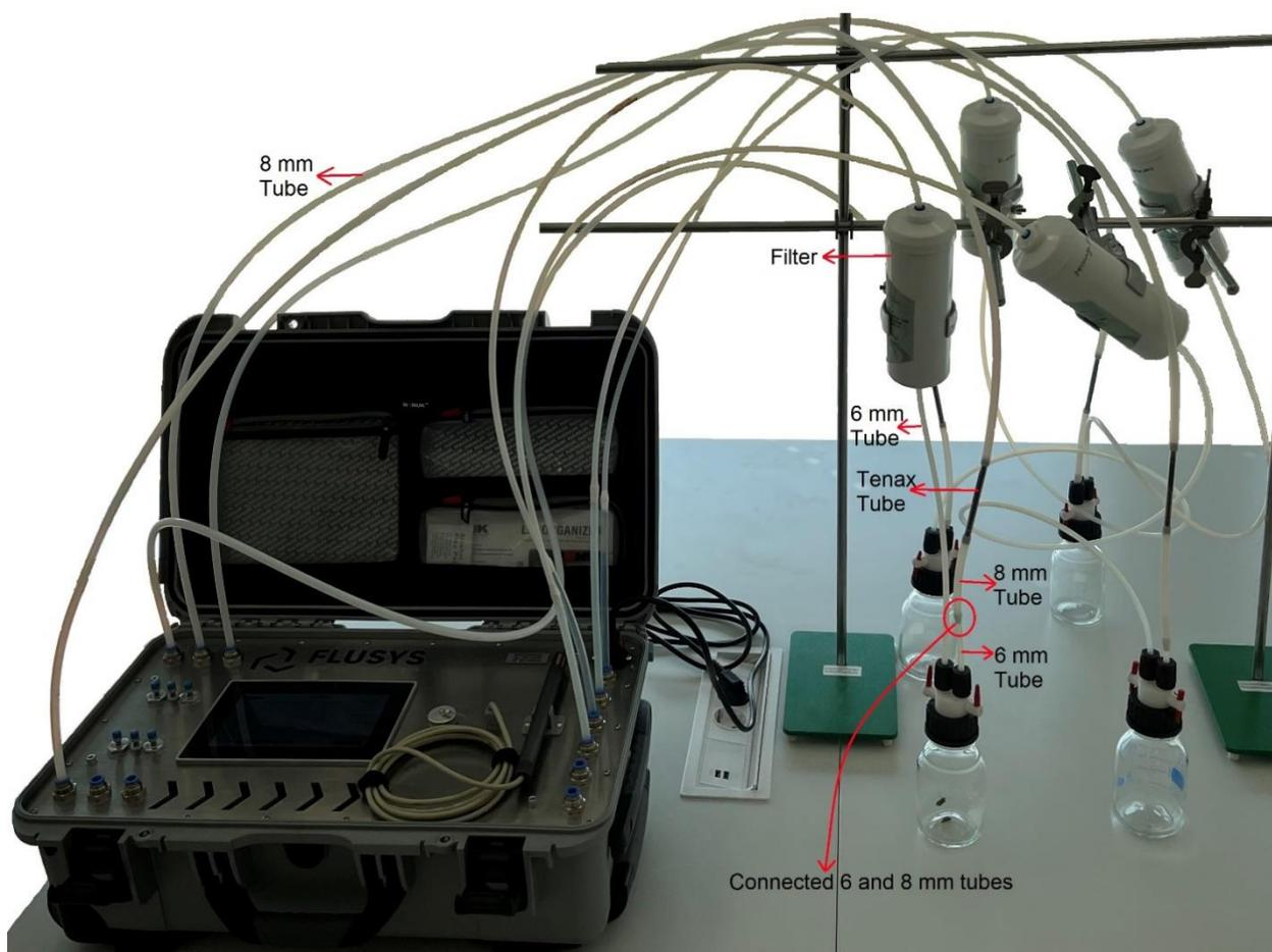
**Figure 3.1:** Preparing the headspace collecting device for collecting VOCs in CLS mode.
