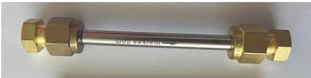
**Figure 3.4:** Tenax tubes sealed with coated brass compression caps.
