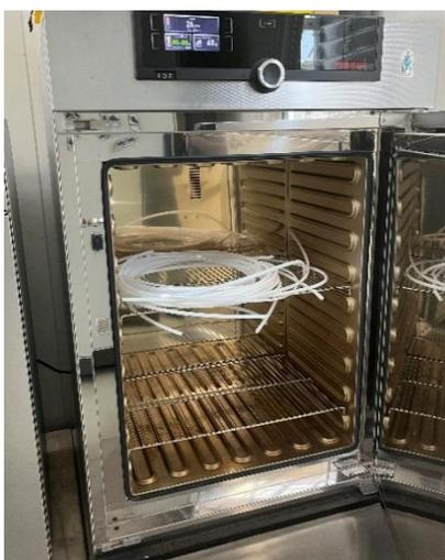
**Figure 3.3:** Cleaned Teflon tubes using an Oven.
