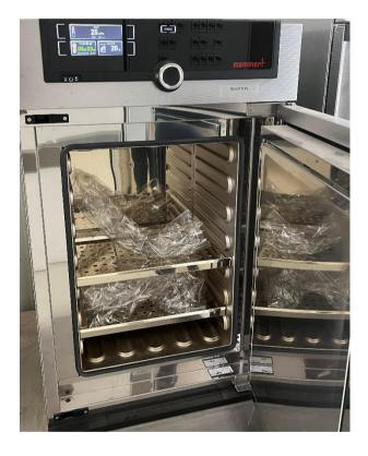
Figure 3.7: The cleaned plastic bag using an oven.
