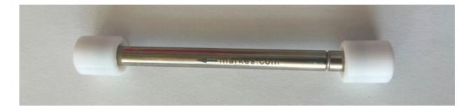
Figure 4.1: Tenax tubes sealed with Teflon caps.
