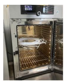
Figure 3.3: Cleaned Teflon tubes using an Oven.
