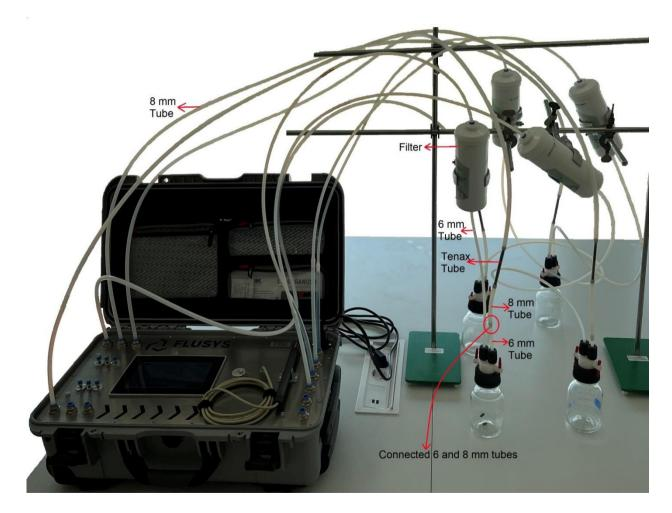
Figure 3.1: Preparing the headspace collecting device for collecting VOCs in CLS mode.
