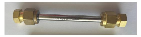
Figure 3.4: Tenax tubes sealed with coated brass compression caps.
