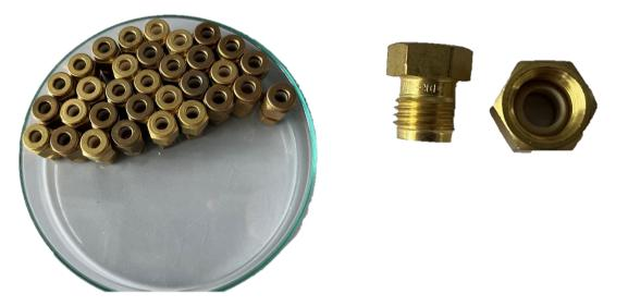
Figure 3.5: Unscrewed Coated brass compression caps (right). The unscrewed caps screwed together again, and prepared for heating in an oven (left).
